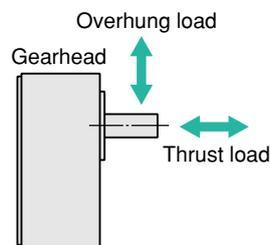
● Overhung Load.....  $W = \frac{K \times T \times f}{\gamma}$
