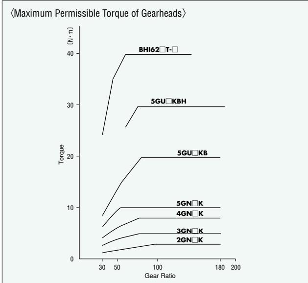
**Example:** If induction motor **4IK25GN-CWE** is combined with gearhead **4GN100K**, the output torque is... The rated torque of motor **4IK25GN-CWE** is 205mN·m. The gearhead output torque is calculated using the equation on the previous page.
