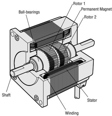
Motor Structure Diagram 1: Cross-Section Parallel to Shaft
