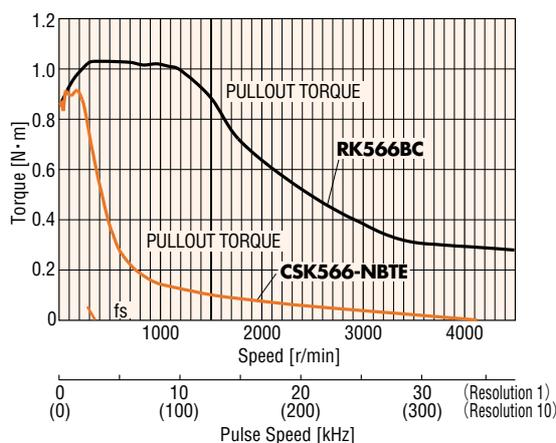
Comparison of characteristics of AC input unit and DC input unit
