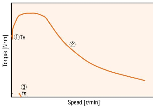
Speed – Torque Characteristics
