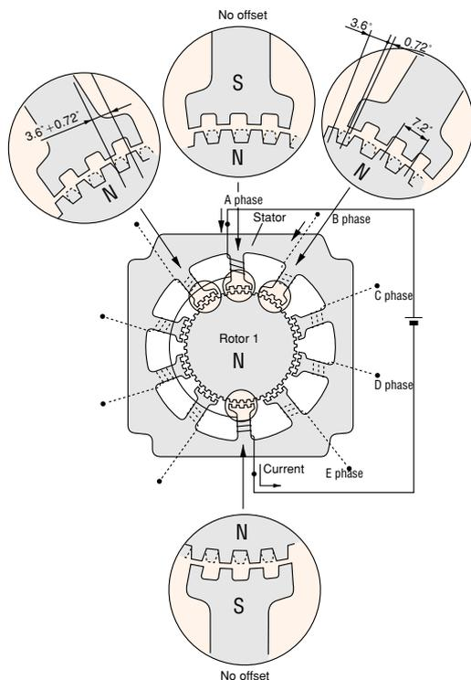
When phase A is excited, its poles are magnetized south and attract the teeth of rotor 1, which are magnetized north, while repelling the teeth of rotor 2, which are magnetized south, which balances it to a stop. The teeth of the phase B poles, which are not excited, are misaligned with the south-polarized teeth of rotor 2 so they are offset by  $0.72^\circ$ .
