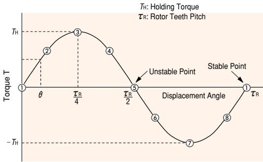
Angle - Torque Characteristics
