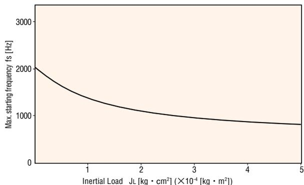
Inertial Load-Starting Frequency Characteristics
