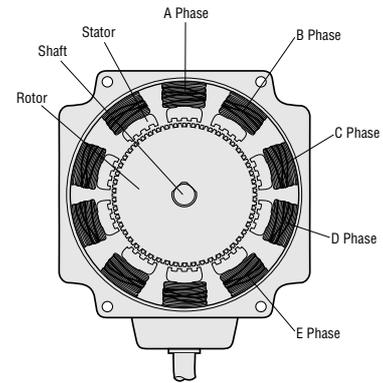
Motor Structure Diagram 2: Cross-Section Perpendicular to Shaft
