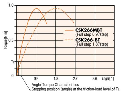
Angle - Torque Characteristics
