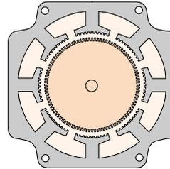
Cross-Section Perpendicular to Shaft
