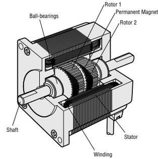
Structure of the 2-Phase High-Resolution Stepping Motor (0.9° per step)
