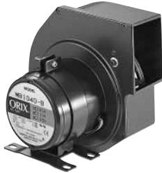
For all the blowers except **MB520** and **MB630**, h2 is longer than h1, therefore, a pedestal must be used when mounting the blower so that the casing does not touch the surface to which the fan is fixed.
