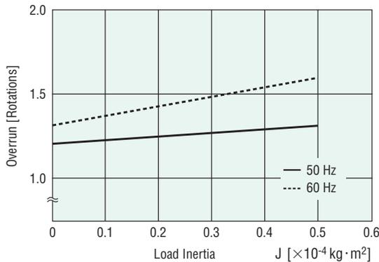
Refer to the braking characteristics curve as a reference value representing the average overrun.
